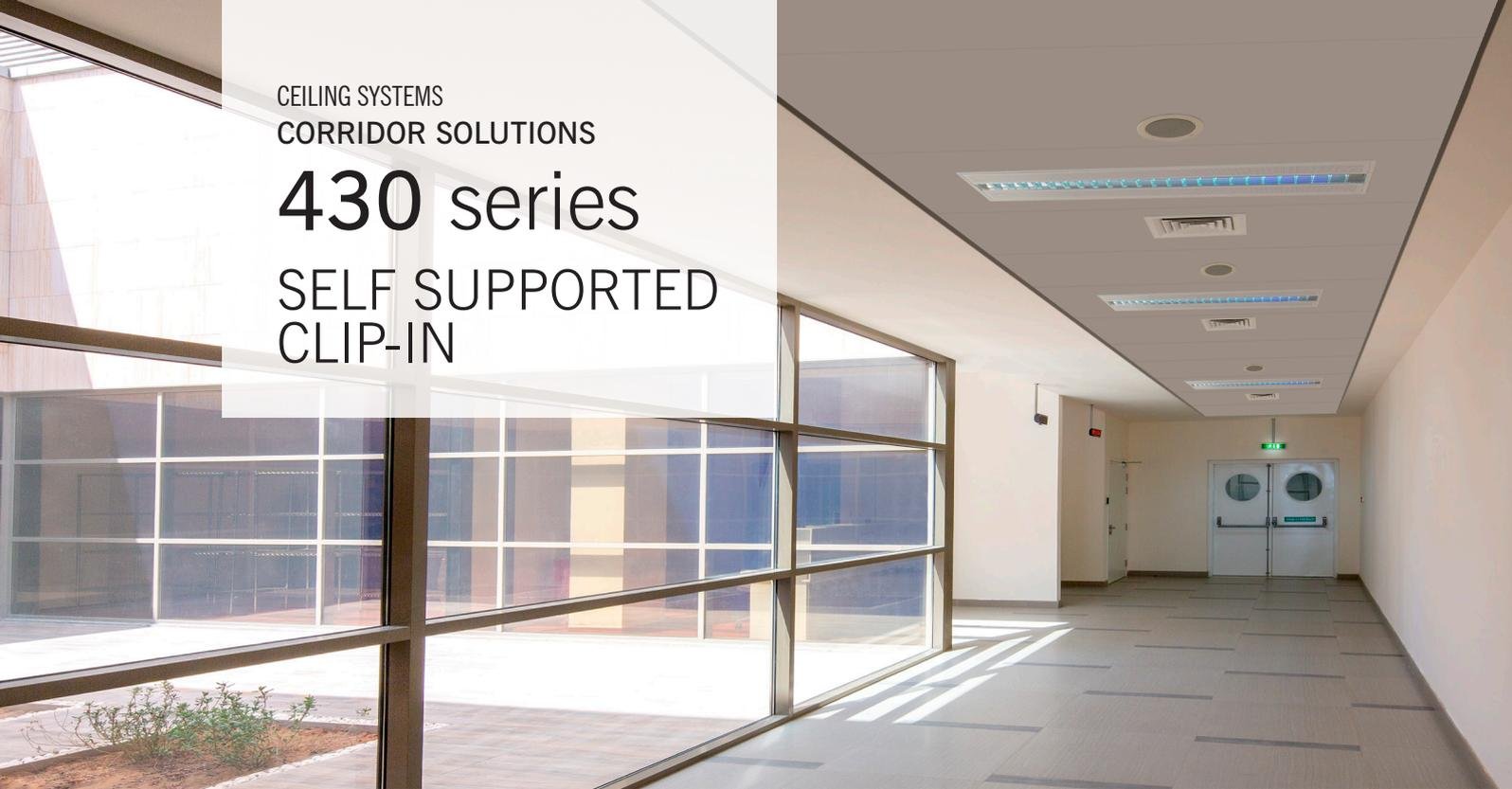
A clip-in type self-supported ceiling for corridor solutions. Modular ceiling panels clipped into concealed 'Z' profile. Fully demountable with downward accessibility using panel removal access key tool. Easy accessibility to ceiling void without any intermediate support. Offered in a wide range of sizes, colors & finishes.
